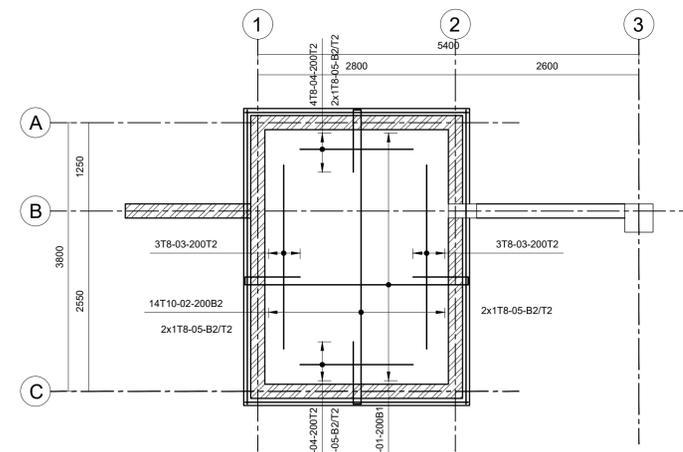
**ROOF FLOOR SLAB RC DETAILS**
