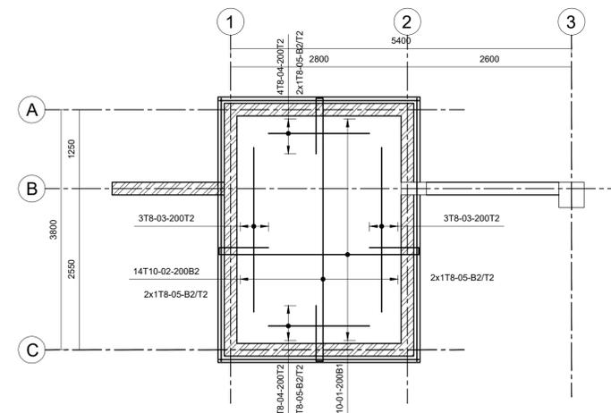
**ROOF FLOOR SLAB RC DETAILS**
