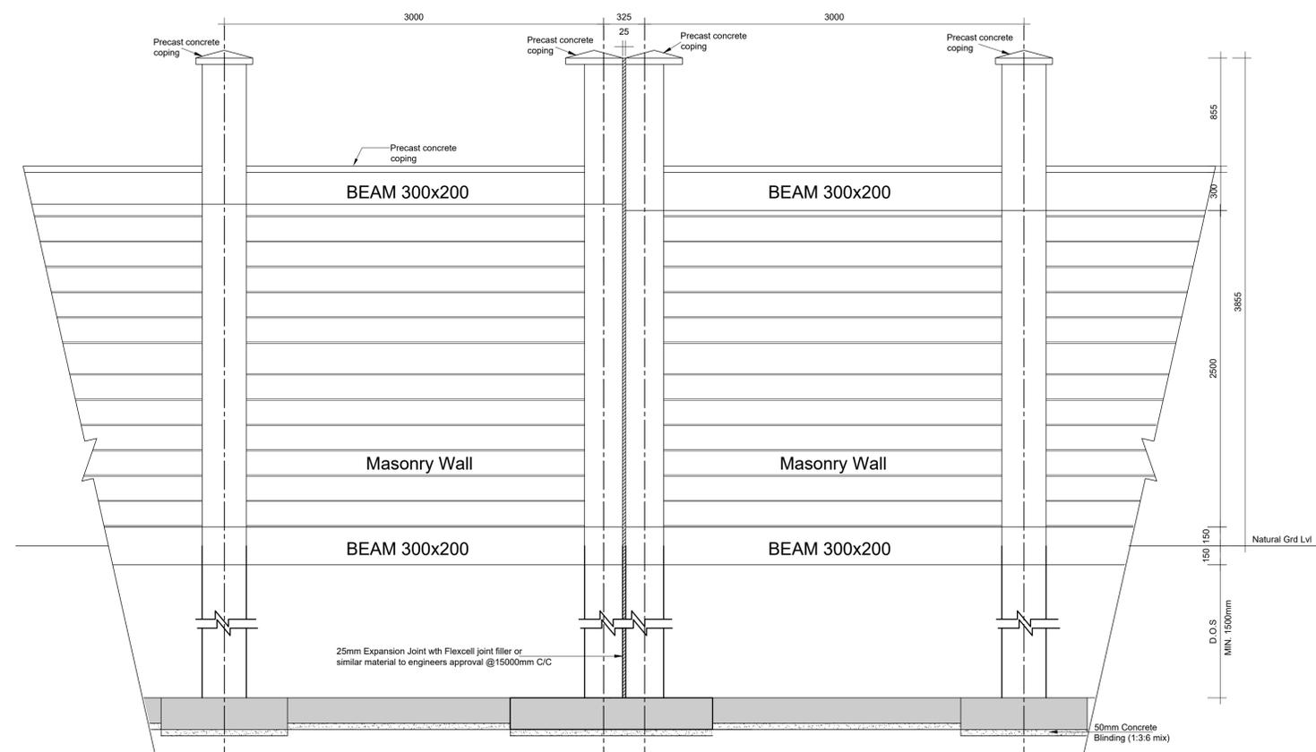
**BOUNDARY WALL ELEVATION (JOINT DETAIL)**
